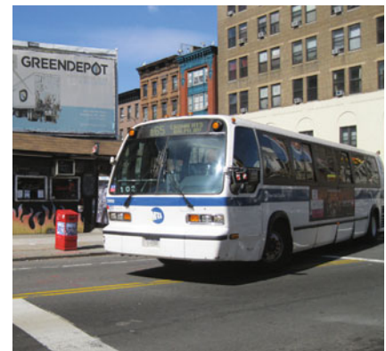
At this intersection, a frequent bus route requires a tight right turn. A recessed stop line paired with a "stop here" sign is used so the bus can complete its turn in one maneuver.
