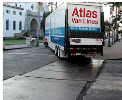
Large trucks infrequently require access to local streets. These vehicles may use opposite lanes to complete the turn.
